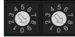
Example: Rotary Switch showing ID No. 99.
