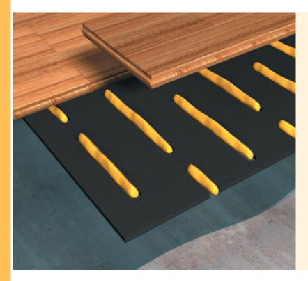
With the moisture regulator and Primer **Sika**<sup>®</sup> **Primer MB** and the Sika wood floor bonding systems, you can make up for delays and eliminate the normal 4 to 6 weeks waiting time.
