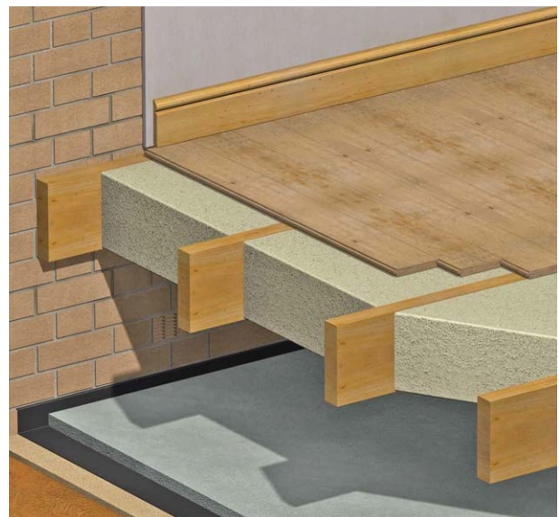
Figure 03: insulating / refurbishing ground floors
